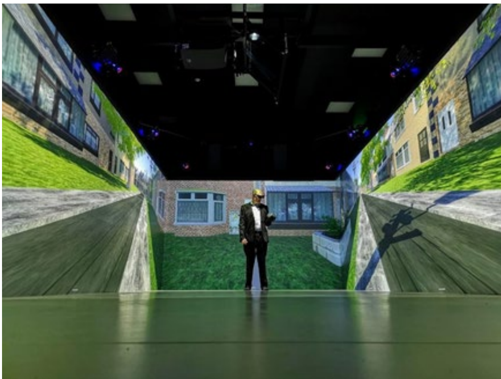
Figure 13 The HIKER pedestrian simulator.
