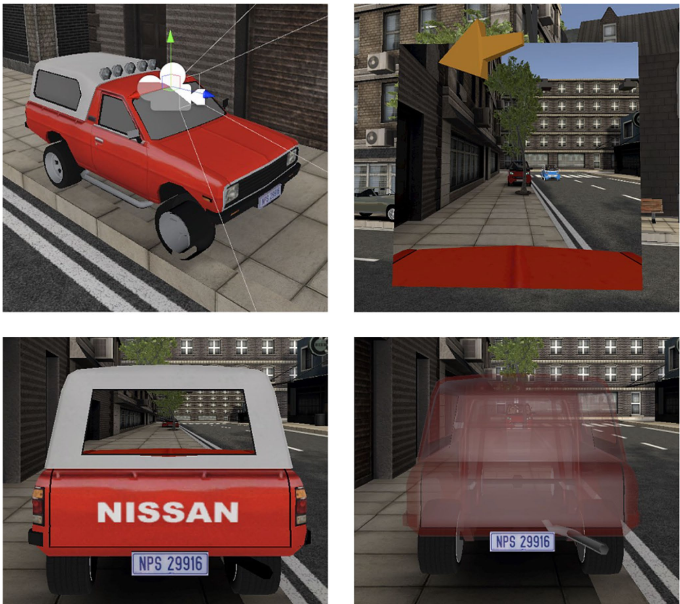
Fig. 6 Top left: Windscreen camera placement. Top right: Close-up view of the VideoHead+ concept. Bottom left: Close-up view of the VideoSeeThrough concept. Bottom right: Close-up view of the TransparentVehicle concept
