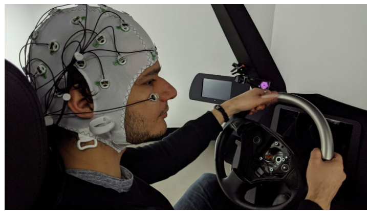
Figure 8 A 32-channel active electrode EEG system that will be used in driving simulator studies at Ulm University
