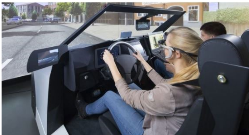
Figure 5 Fixed-base driving simulator with 190° field of vision, available at the Ulm University
