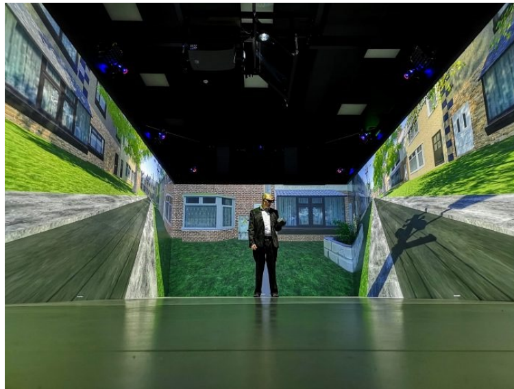
Figure 6 The Highly Immersive Kinematic Experimental Research (HIKER) lab, which is the largest 'CAVE-based' pedestrian simulation environment of its type in the world, available at the University of Leeds
