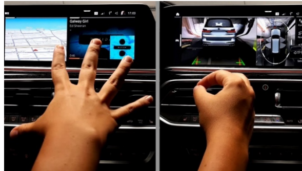
Figure 9 – Use of hand gestures for interaction with HMI, BMW X7 (Cardesign use, 2019)
