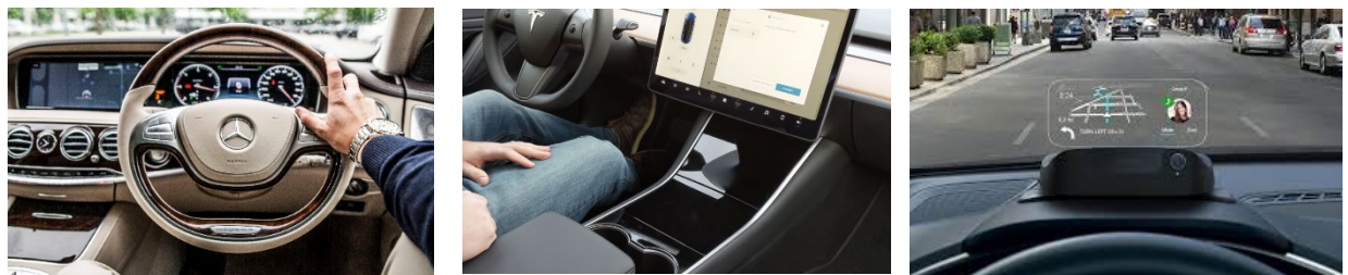
Figure 1 – A typical vehicle dashboard, showing speedometer and tachometer (left, AnyRGB) use of the central console for information (centre, Tesla, 2017), and a Head Up Display (right) for presentation of navigation information in vehicles (Fogelson, 2017)
