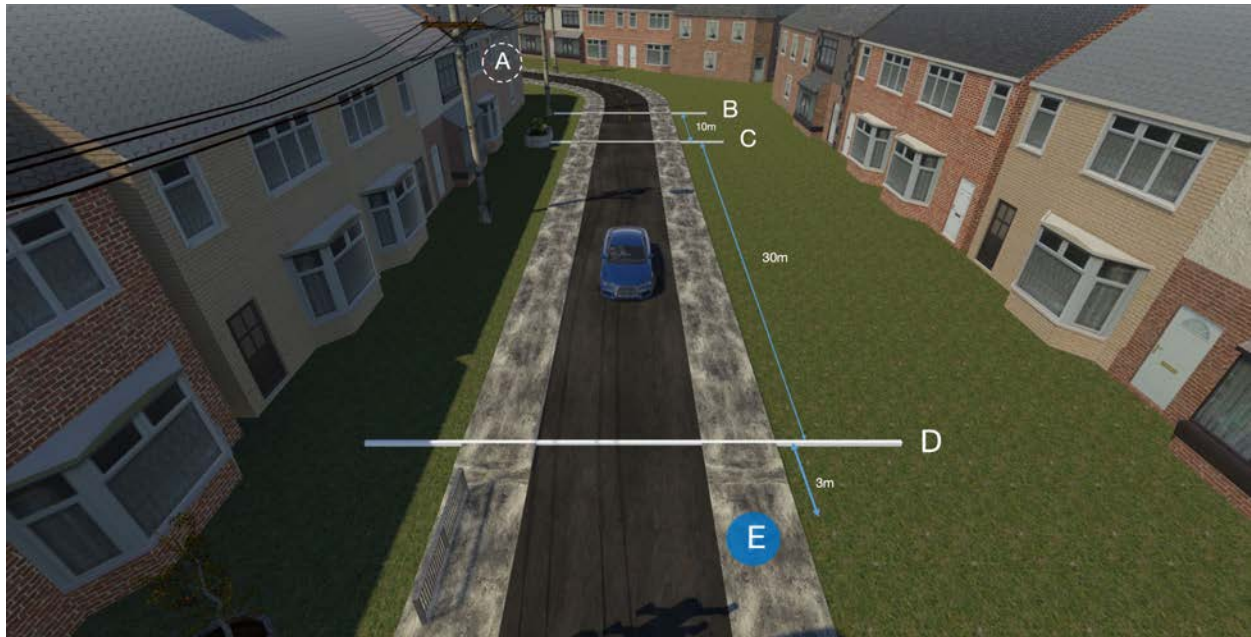
Figure 2. The simulation environment used for the HIKER experiment. Each salient point is demarcated by a label, together with the distance (in metres) between each point. A: spawn point, B: AR interface onset, C: AV deceleration onset, D: stopping point, E: participant location. Image adapted from Tabone et al. (2023).
